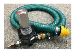
THE NOAQ PRESSURE GUARD is an accessory to the NOAQ Tubewall. It makes it possible to connect the tubewall to a compressor or a compressed-air installation. The device includes a pressure reducing valve that maintains the air pressure in the tubewall within the recommended interval, close to 7 kPa (70 mbar or 1 psi).
