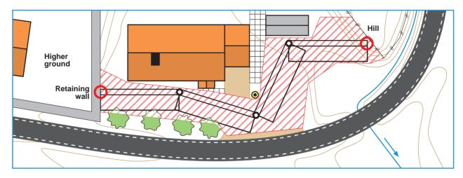
If no secure ending points are found near the object the tube wall will have to encircle it. If other threatened objects are too close (like terrace houses) the tube wall may have to be extended to protect the whole group of objects.
