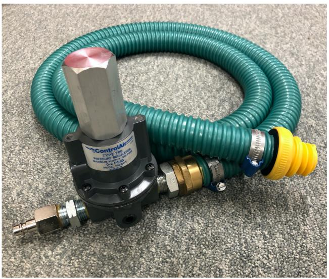
The NOAQ Pressure Guard is an accessory to the NOAQ Tubewall. It makes it possible to connect the tubewall to a compressor or a compressed-air installation. The device includes a pressure reducing valve that maintains the air pressure in the tubewall within the recommended interval, close to 7 kPa (70 mbar or 1 psi). If an air leak should occur the pressure guard will immidiately restore the pressure.
